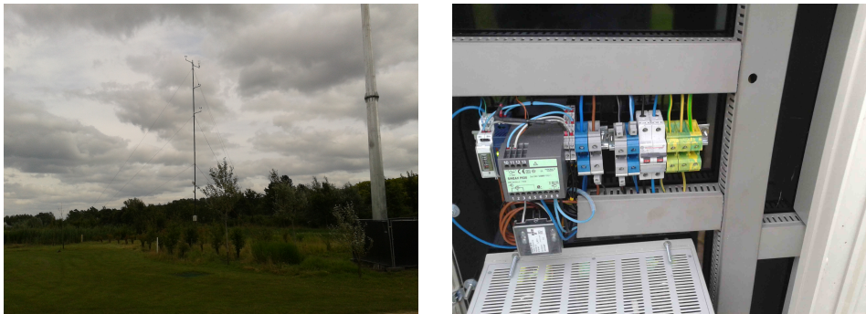
Figure 5.23: Wind measurement mast (left) and power measurements (right) for the HY5kW wind turbine.
