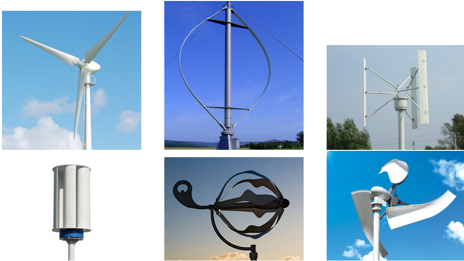
Figure 2.1: Database categories: horizontal-axis (top left), vertical-axis (top middle and top right) and ‘other’ types (bottom) of wind turbines.
